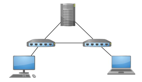
A device known as a **controller** instructs **forwarding devices** on how to forward network traffic
