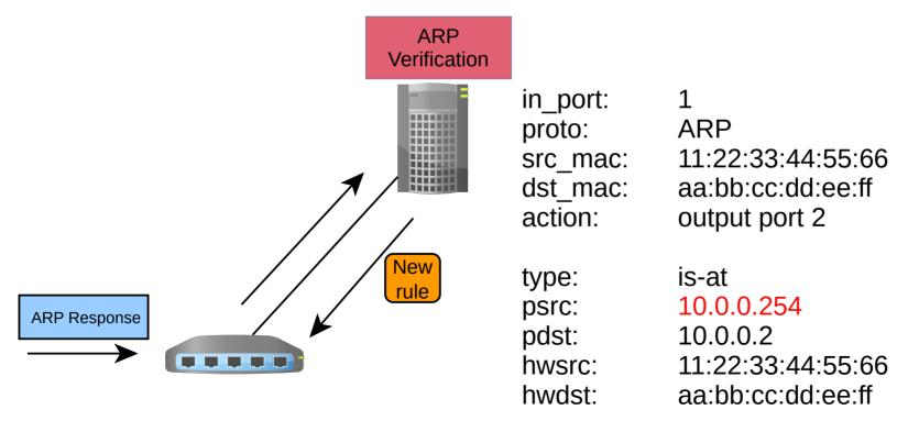
The modified ARP response can be piggyback on the existing forwarding rule so the controller will never observe it
